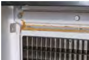
Ice machine without LuminIce II
