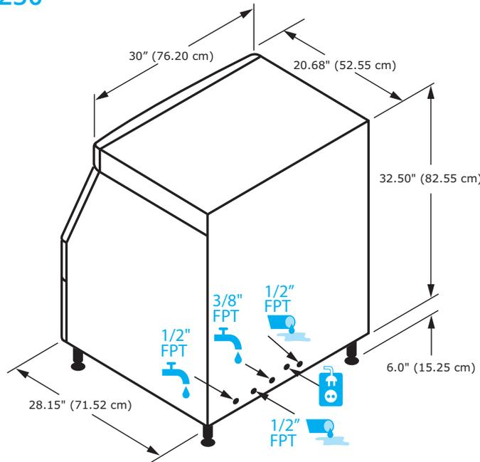
**Installation Note:** Recommended clearance for top, sides, and back is 5" (127 cm). However, there is no minimum clearance required.
