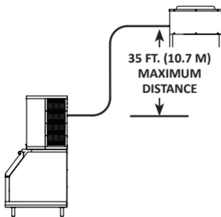
**35 ft. (10.7 m) Rise:** The maximum distance the Condenser or Condensing Unit can be above the ice machine.
