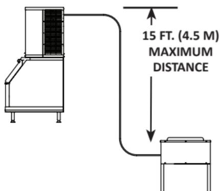
**15 ft. (4.5 m) Drop:** The maximum distance the Condenser or Condensing Unit can be below the ice machine.
