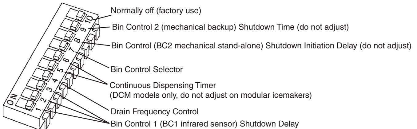
**2. BC1 (Infrared Sensor) Shutdown Delay (S1 dip switch 1, 2, 3)**
