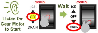
**i** The icemaker might make a noise/squealing when first started due to scale removal from auger/evaporator. This is normal in bad water conditions and will subside after 20 minutes.
